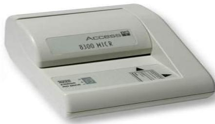
MICR input device is generally used in banks because of a large number of cheques to be processed every day. The bank's code number and cheque number are printed on the cheques with a special type of ink that contains particles of magnetic material that are machine readable. This reading process is called Magnetic Ink Character Recognition (MICR). The main advantage of MICR is that it is fast and less error prone.
